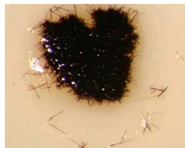
Figure 2. Long, needle-shaped dark brown single crystals of \text{Ag}(\text{SO}_3\text{F})_2 grown from \text{HSO}_3\text{F} as a product of the reaction [Equation (3)] over several days, intergrown in the form of hedgehogs and of larger conglomerates.
